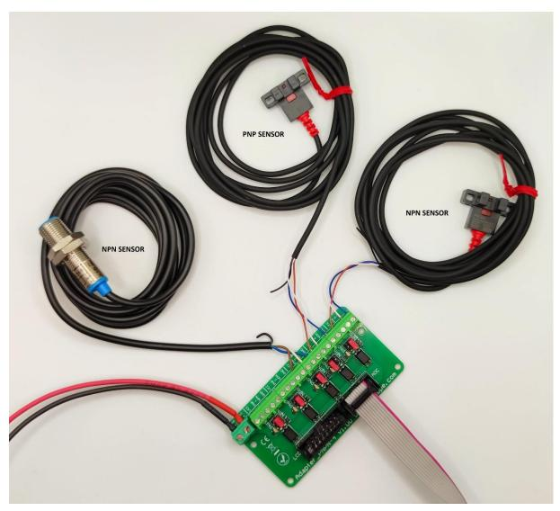
All sensors in the picture have NC leads connected since that is recommended in most use cases. The white signal wire is connected to the appropriate input and jumper is set. For connection with PoKeys57CNC the ADC connector is used.
